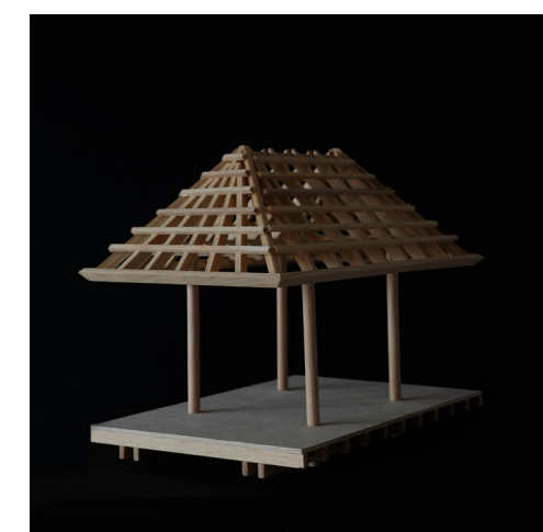
structural principle: stone - column - floor - roof
