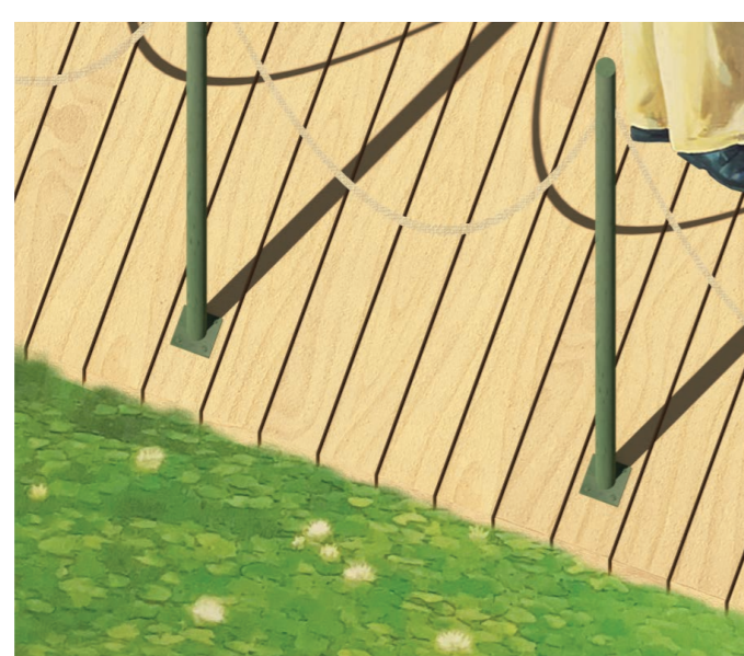
duckboards - timber flooring; metal plugs and post for protection; rope handrail
